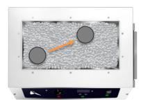
Note: Do not place frozen vessels adjacent to the temperature probe located in the front, right corner of the tank. This will cause the probe to register the chilled temperature of the beads immediately surrounding the frozen samples, potentially causing the bead bath to raise the overall bath temperature.
