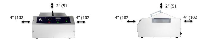
4 inches (102 mm) of clearance is required on the sides and back.
